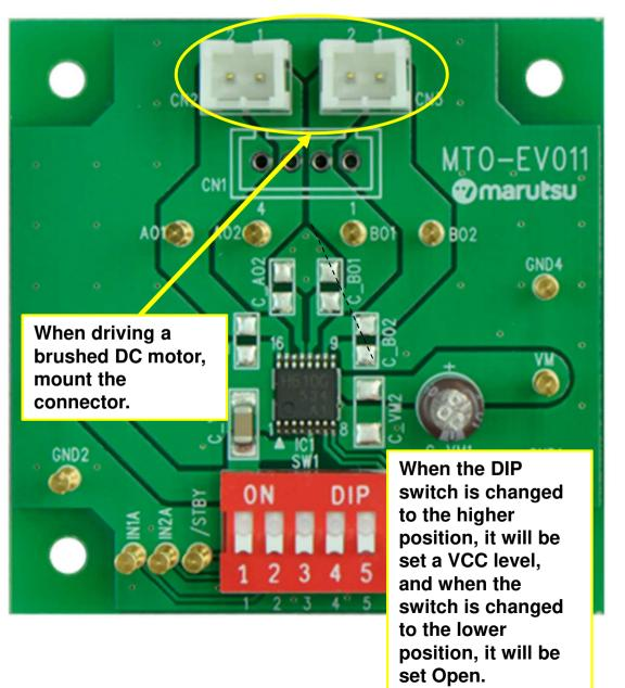
This evaluation board has a DIP switch (SW) so that the operation setting of the TC78H621FNG can be set without the external signal input.
