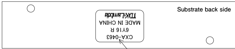
Example of label marking Product name, Lot No., Country of origin, TDK-Lambda logotype
