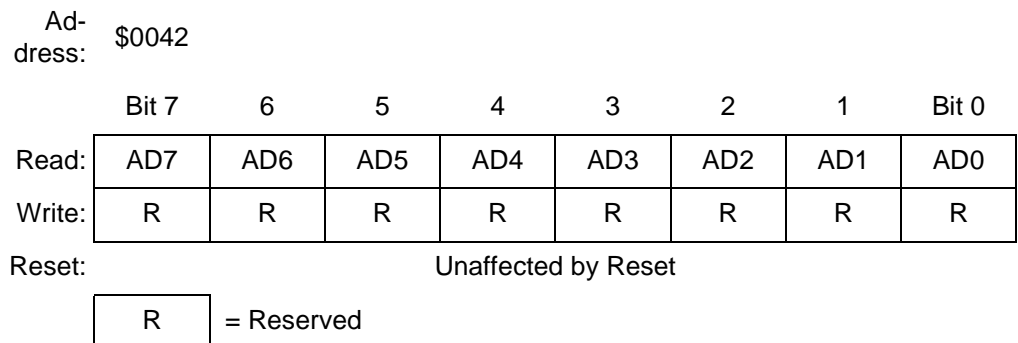
Figure 18-7. ADC Data Register Low (ADRL) Right Justified Mode
