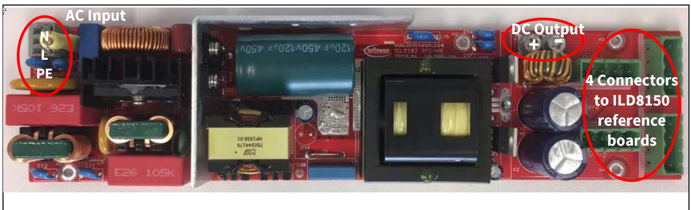
Figure 1 ICL5102 320 W CV reference board – top side
