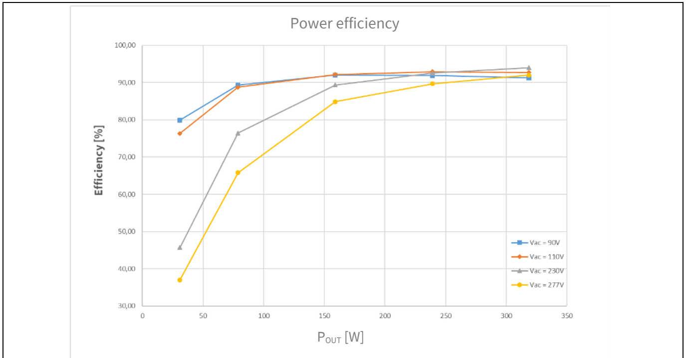
Figure 16 ICL5102 320 W reference board power efficiency measurement
