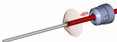
Completely widen shield braid. Push seal insert (2) under shield braid
