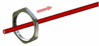
Place counter nut (1) on cable
