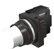
30mm BlackMax, Epoxy Coated Corrosion Resistant Complete Metal Unit Illuminated Indicator Light Full Voltage type, 6V AC/DC Incandescent Lamp, BA9s Plastic Lens, White UL Listed, CSA Certified NEMA 1,3,3R,4,4X,12,13 & Automotive Standards
