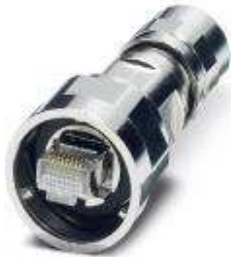
RJ45 connector, IP67, with bayonet locking, metal housing, CAT5e, 8-pos., IDC connection method, for 26 AWG 7-wire conductors, for 5.0 mm ... 10.0 mm cable diameter
