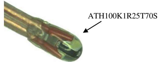
Figure 4.3. Tubing Ledged Sealed Thermistor Head Photo
