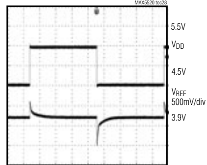
REFERENCE LINE-TRANSIENT RESPONSE ( V_{REF} = 3.9V )
