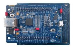
Plug the HSMC Interconnect Board (CYUSB3ACC-006) into the Altera® FPGA board (The Altera FPGA board is not part of this kit)
