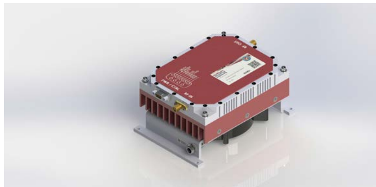
PA Module w/ Fan-Cooled Heatsink
