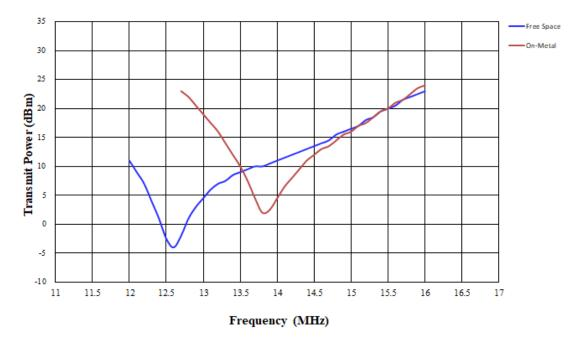
\*HF sensitivity shown in the figure is measured by Voyantic Tagformance HF Loop Antenna C60 on 15\*15mm steel plate. Actual sensitivity performance is subject to the environment in practice.
