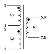
Application of the transformer allows for the leadwires between terminals 5&6 and 7&8 to solder bridge.
