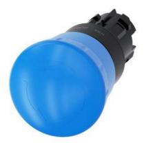
Mushroom pushbutton, 22 mm, round, plastic, blue, 40 mm, positive latching, acc. to EN ISO 13850, rotate-to-unlatch, with laser labeling, inscription or symbol Customer-specific selection with SIRIUS ACT configurator (CIN)
