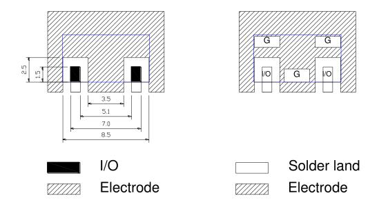
Shielding case layout guide (MIN)
