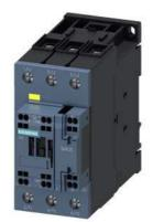
power contactor, AC-3e/AC-3, 51 A, 22 kW / 400 V, 3-pole, 21-33 V AC/DC, 50/60 Hz, with integrated varistor, auxiliary contacts: 1 NC, main circuit: screw terminal, control and auxiliary circuit: spring-loaded terminal, size: S2, F-PLC-IN
