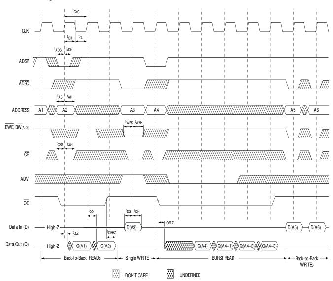
19. <u>The</u> data bus (Q) remains in tri-state following a WRITE cycle unless a new read access is initiated by ADSP or ADSC. 20. <u>GW</u> is HIGH.
