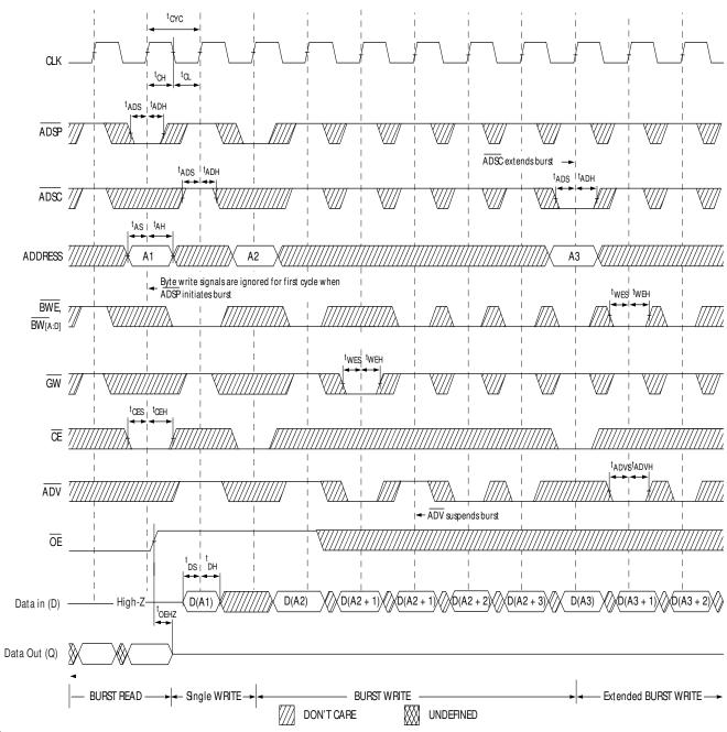
18. Full width write can be initiated by either  $\overline{\text{GW}}$  LOW; or by  $\overline{\text{GW}}$  HIGH,  $\overline{\text{BWE}}$  LOW and  $\overline{\text{BW}}_{[A:D]}$  LOW.
