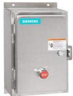
Non-reversing motor starter, Size 0, Three phase full voltage, Solid-state overload relay, OLR amp range 0.25-1A, 208VAC 60Hz coil, Non-combination type, Encl. type 4X 304 S. Steel, Water/dust tight noncorrosive, Standard width enclosure
