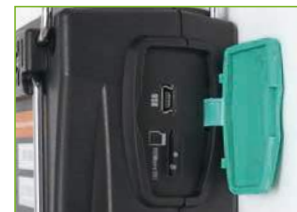
USB port and Micro SD card for software update and data output
