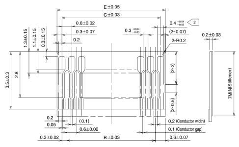
Note 1 Polyimide and thermal hardening glue are a recommendation for the stiffener.
