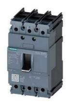
circuit breaker 3VA5 UL frame 125 breaking capacity class H 65kA @ 480 V 3-pole, line protection TM210, FTFM, In=15A overload protection Ir=15A fixed short-circuit protection Ii=20 x In UL489 SB (naval), 50 deg. cel. nut keeper kit on both sides
