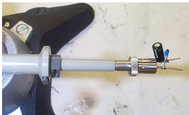
Figure 95 – Oscilloscope Probe with Probe Master ( www.probemaster.com ) 4987A BNC Adapter. (Modified with wires for ripple measurement, and two parallel decoupling capacitors added)
