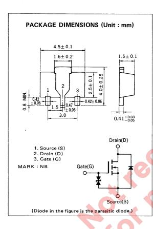
The 2SK1483 is an N-channel vertical type MOS FET switching device which can be directly driven from an IC operating with a 5 V single power supply. The device features low ON-state resistance and outstanding switching characteristics and thus is ideal for driving actuators such as motors, solenoids, and relays.
