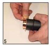
**Step 6:** Apply adhesive copper tape completely around the cable core shields. Both inner and outer shield will be in full contact with tape. Both drain wires will be outside the copper tape.
