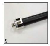
**Step 10:** Using 2.0" box wrenches, fully tighten down the connector until snug. Go one-quarter turn to completely tighten. NOTE: It is recommended to use an additional stress boot at the cable to connector interface. A shrink boot, silicone tape or strong electrical tape will add strength.
