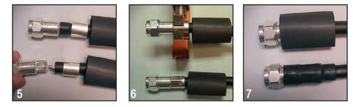
**Step 5**: Slide the connector over the end of the core and push it up to the end of the jacket. Rotate the connection back and forth in a clockwise-counter clockwise motion in reference to the axis of the cable until the back of the connector works its way under the end of the jacket. Now push the connector onto the cable with some back and forth motion until it stops.
