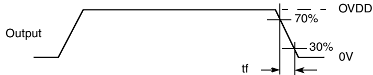
Figure 7. Definition of Timing for Standard and Fast-Mode
