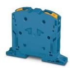
High-current terminal block, nom. voltage: 1000 V, nominal current: 232 A, connection method: Power-Turn connection, 1 level, cross section: 25 mm² - 95 mm², mounting type: direct screw connection, color: blue
