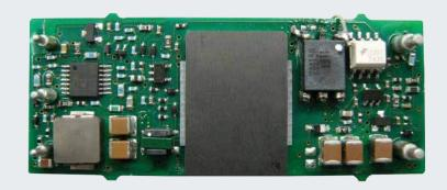
Advanced Energy's Artesyn IBC04-36S12 is the latest wide-range input isolated DC-DC converter specifically designed to supply non-isolated converter architectures. It operates from an ultra-wide input range of 18 Vdc to 60 Vdc and provides a regulated output voltage of 12 V. The output is rated to a power level up to 50 W.
