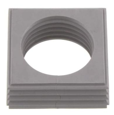
Seal, Mounting type: Plug in, Length x width: 42.8 mm, Max. cable diameter: 32 mm, IP 66, Colour: Grey
