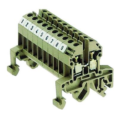
Feed-through terminal/block variant, Screw connection, Mounting type:Mounting rail TS 35/7.5 and TS 32, Rated cross-section: 4 mm², Colour: Beige
