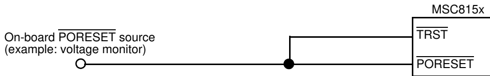
Figure 35. Reset Connection in Functional Application
