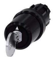
Key-operated switch BKS, 22 mm, round, plastic, special lock, with 2 keys, 3 switch positions I>O<II, momentary contact on the left, latching on the right, actuating angle 2x45°, 10:30h/12h/13:30h, key removal O, Note: BKS locking systems E1 - E25 supplied without key
