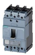
circuit breaker 3VA5 UL frame 125 breaking capacity class M 35kA @ 480 V 3-pole, line protection TM230, FTAM, In=110A overload protection Ir=110A fixed short-circuit protection Ii=5...10 x In UL489 SB (naval), 50 deg. cel. cable connection on both sides
