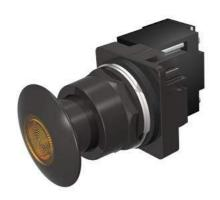
30mm BlackMax, Epoxy Coated Corrosion Resistant Complete Metal Unit Illuminated Push-Pull Operator Transformer type, 600V AC LED Lamp Mushroom Head Cap Small 1 3/4" (44.5 mm) Metal, Black with Amber Lens 3 Position Pull-Momentary/Push-Maintained UL Listed, CSA Certified NEMA 1,3,3R,4,4X,12,13 & Automotive Standards
