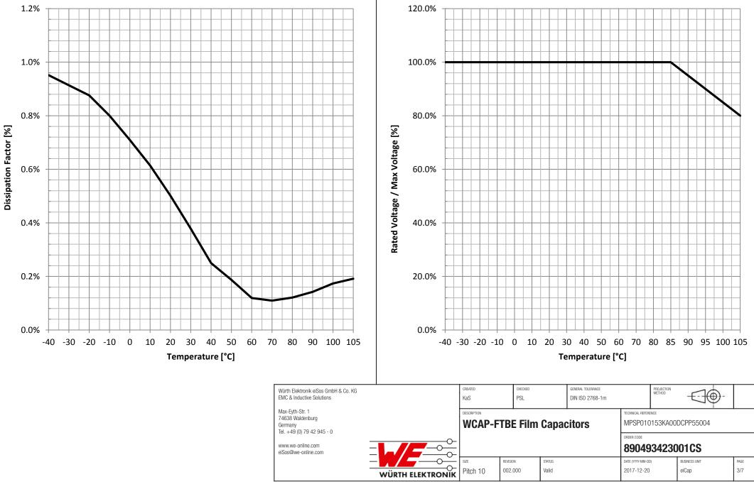
**Rated Voltage vs. Temperature:**
