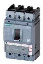
circuit breaker 3VA5 UL frame 250 breaking capacity class H 65kA @ 480 V 3-pole, line protection TM210, FTFM, In=70A overload protection Ir=70A fixed short-circuit protection Ii=10 x In UL489 SB (naval), 50 deg. cel. cable connection on both sides
