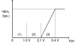
\*: The maximum ON duty is  $T_{ON} = 95\%$  (typ.) when VSP = 5.4 V (typ.). Example: If fosc = 5 MHz, then ON time = 48  $\mu$ s (typ.) (fc = 19.8 kHz) If fosc = 4 MHz, then ON time = 60  $\mu$ s (typ.) (fc = 15.9 kHz)
