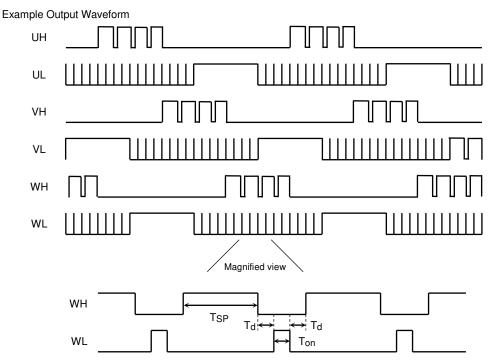
T<sub>SP</sub>: Variable depending on the VSP (the figure above being applicable when VSP = 5.4 V (typ.)); Ton = 18/fosc; Td = 18/fosc
