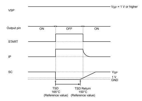
Note: The TSD circuit is not intended to provide protection against all abnormal conditions. Therefore, the TB6588FG should exit the abnormal state immediately after the TSD circuit is enabled.
