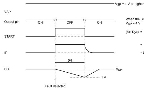
When the SC pin capacitor = 0.47  $\mu\text{F}$  and  $V_{SP}$  = 4 V
