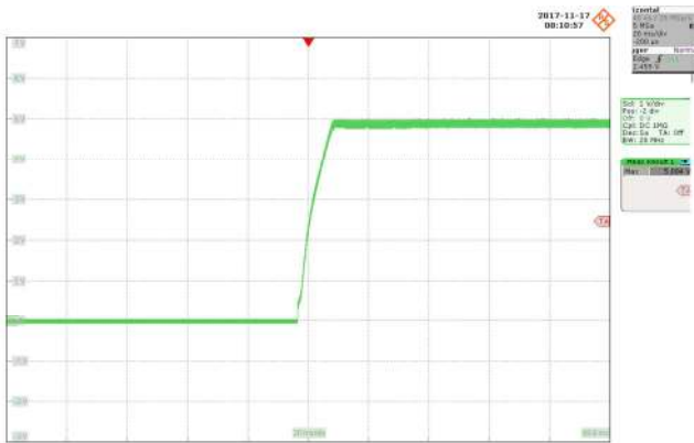
Figure 24 – 85 VAC Input, Full Load. V_{OUT} , 1 V / div., 20 ms / div.
