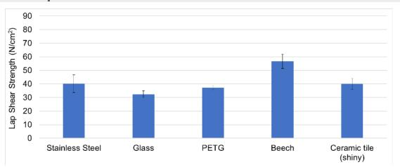
The graph was generated by testing Sugru® on a range of materials according to ASTM D 1002. Samples of lap shear joints with 2 mm thickness, 25.4 mm width and 12.7 mm overlap were tested after 24 hrs curing at 25°C and 50% relative humidity.
