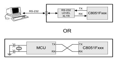
Figure 16.3. UART Interconnect Diagram
