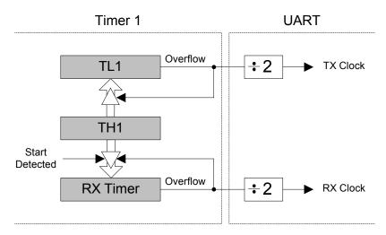
Figure 16.2. UARTO Baud Rate Logic
