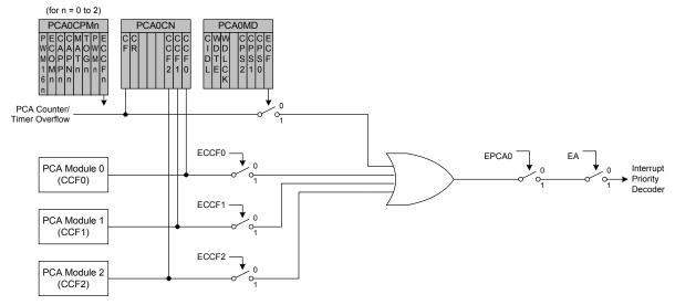
Figure 19.3. PCA Interrupt Block Diagram
