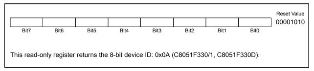
Figure 20.2. DEVICEID: C2 Device ID Register
