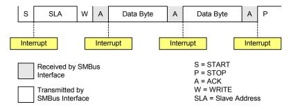
Figure 15.8. Typical Master Transmitter Sequence
