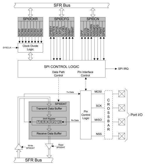
Figure 17.1. SPI Block Diagram
