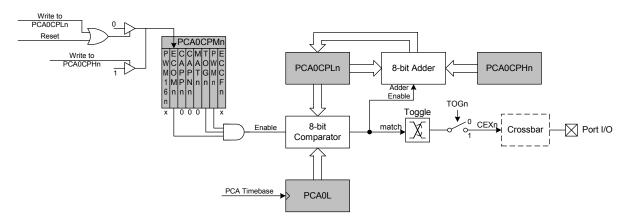
Figure 19.7. PCA Frequency Output Mode
