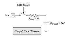
Figure 5.4. ADC0 Equivalent Input Circuits
