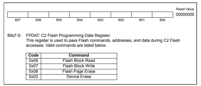
Figure 20.5. FPDAT: C2 Flash Programming Data Register
