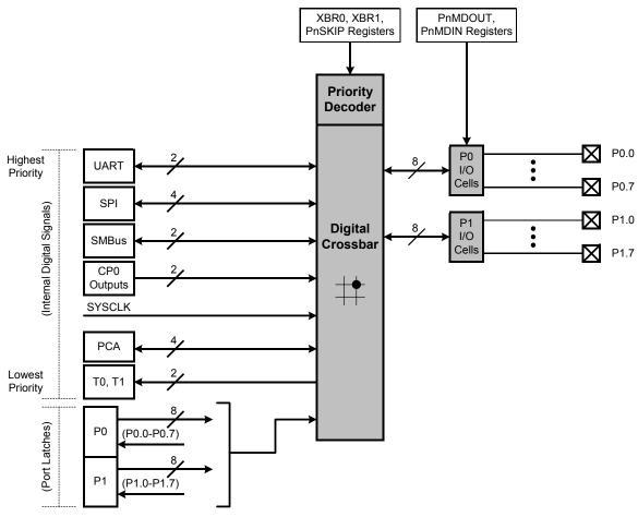
Figure 14.1. Port I/O Functional Block Diagram
