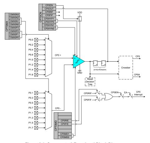
Figure 8.1. Comparator Functional Block Diagram
