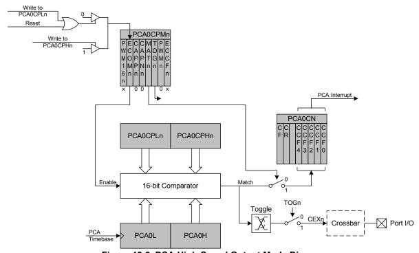
Figure 19.6. PCA High-Speed Output Mode Diagram
