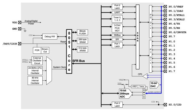
Figure 1.1. C8051F330 and C8051F330D Block Diagram
