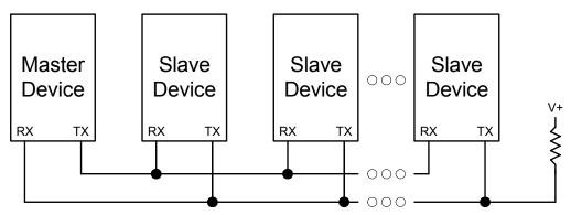
Figure 16.6. UART Multi-Processor Mode Interconnect Diagram
