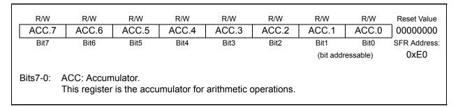
Figure 9.7. ACC: Accumulator
