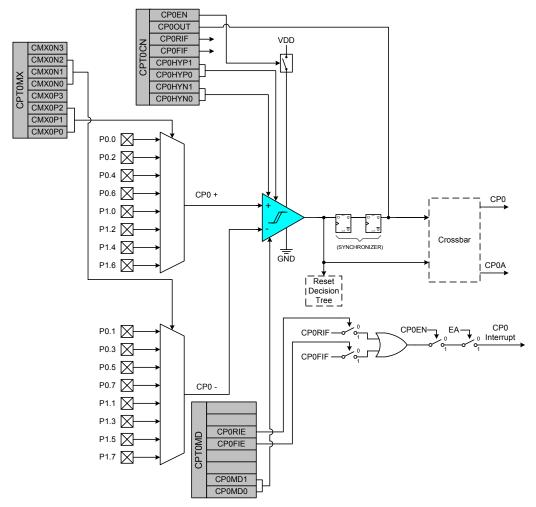
Figure 1.11. Comparator Block Diagram
