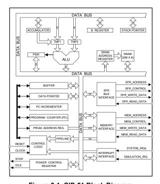
Figure 9.1. CIP-51 Block Diagram
