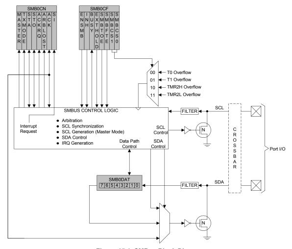
Figure 15.1. SMBus Block Diagram
