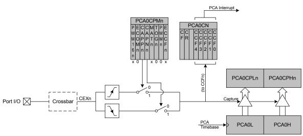
Figure 19.4. PCA Capture Mode Diagram
