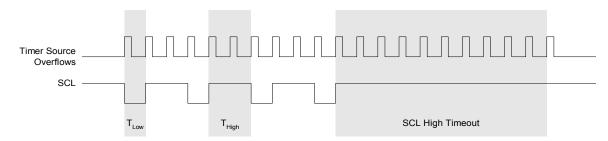
Figure 15.4. Typical SMBus SCL Generation
