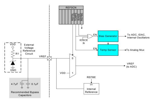
Figure 7.1. Voltage Reference Functional Block Diagram
