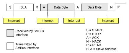
Figure 15.9. Typical Master Receiver Sequence
