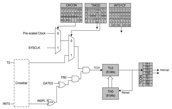
Figure 18.2. T0 Mode 2 Block Diagram
