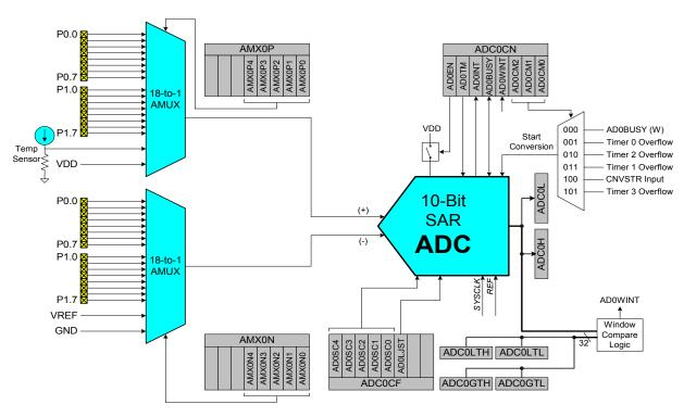
Figure 5.1. ADC0 Functional Block Diagram
