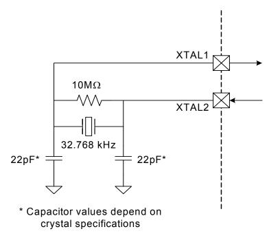
Figure 13.6. External 32.768 kHz Quartz Crystal Oscillator Connection Diagram
