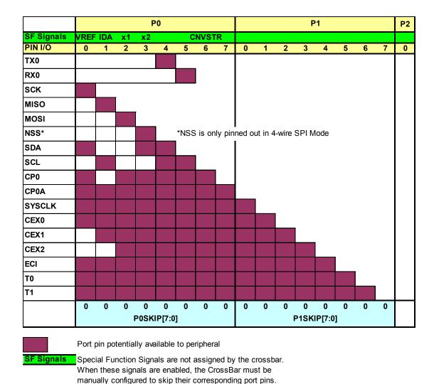
Figure 14.3. Crossbar Priority Decoder with No Pins Skipped
