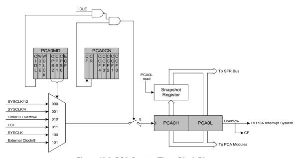
Figure 19.2. PCA Counter/Timer Block Diagram
