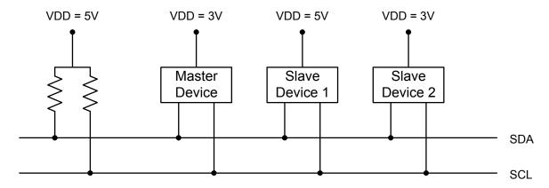
Figure 15.2. Typical SMBus Configuration
