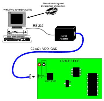
Figure 1.6. Development/In-System Debug Diagram
