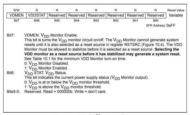
Figure 10.3. VDM0CN: V<sub>DD</sub> Monitor Control
