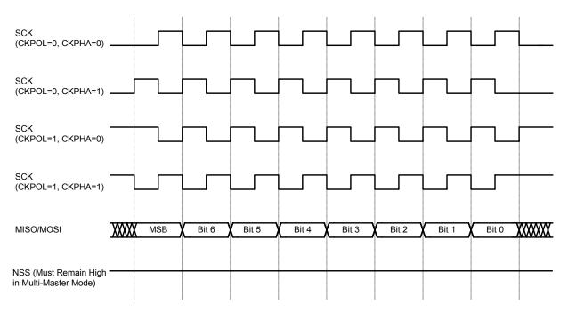
Figure 17.5. Master Mode Data/Clock Timing
