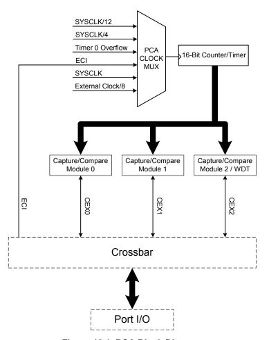
Figure 19.1. PCA Block Diagram
