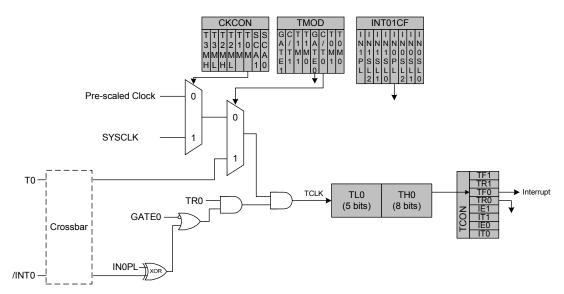
Figure 18.1. T0 Mode 0 Block Diagram
