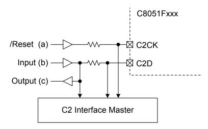
Figure 20.6. Typical C2 Pin Sharing
