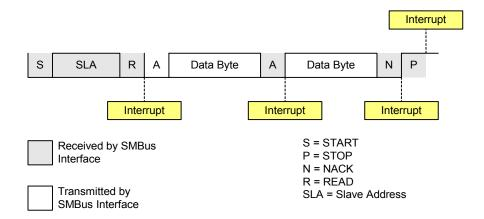
Figure 15.11. Typical Slave Transmitter Sequence
