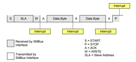
Figure 15.10. Typical Slave Receiver Sequence
