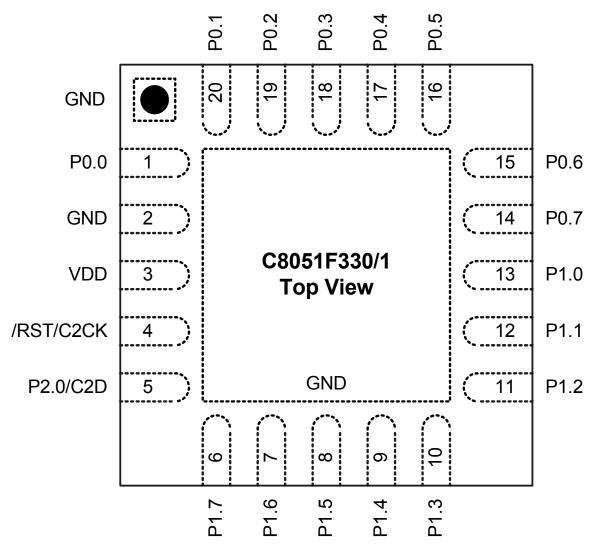
Figure 4.1. MLP-20 Pinout Diagram (Top View)
