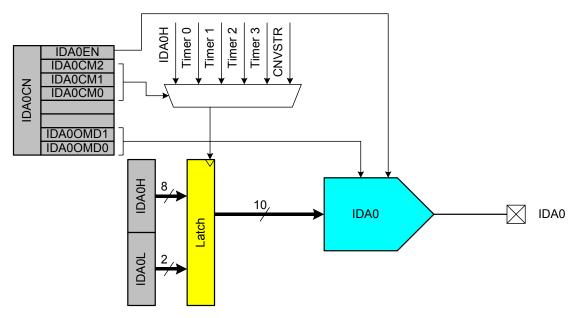
Figure 6.1. IDA0 Functional Block Diagram
