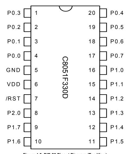
Figure 4.5. DIP-20 Pinout Diagram (Top View)
