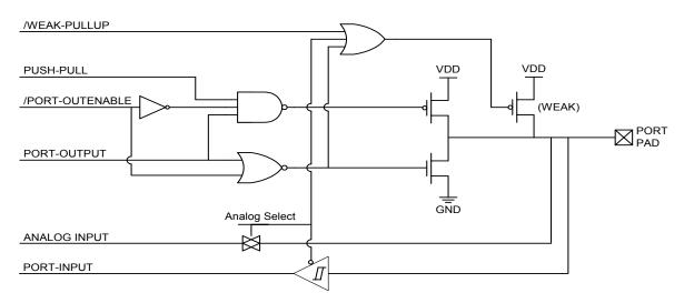
Figure 14.2. Port I/O Cell Block Diagram
