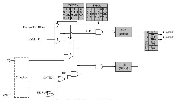
Figure 18.3. T0 Mode 3 Block Diagram
