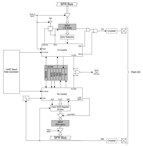
Figure 16.1. UARTO Block Diagram
