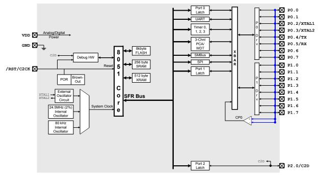
Figure 1.2. C8051F331 Block Diagram
