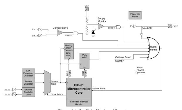
Figure 1.4. On-Chip Clock and Reset
