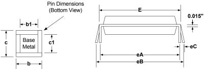
Figure 4.6. DIP-20 Package Drawing
