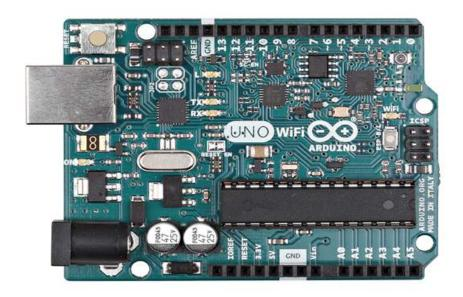
The Arduino UNO WiFi board is based on the ATmega328 and it has an integrated ESP8266 WiFi Module. If you are starting out with Arduino, or starting with IoT, this is the board to get.
