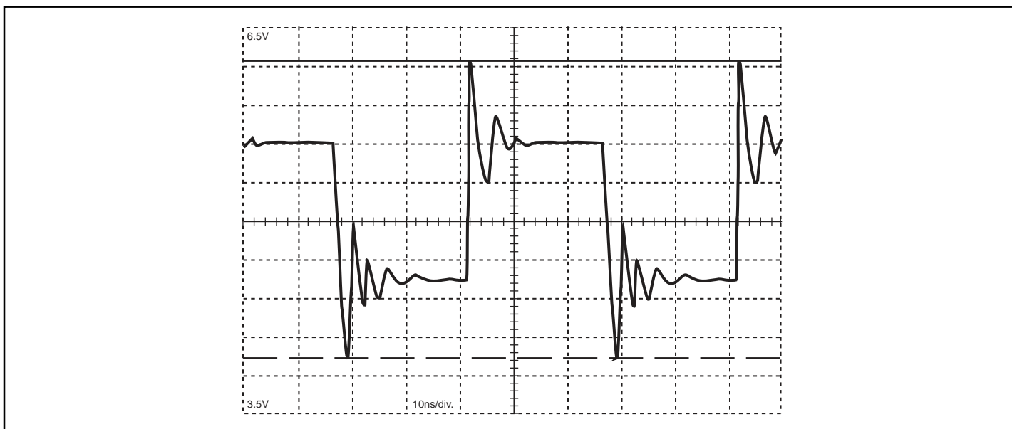
Figure 2. VCX16244 (Vcc = 3.6V) output after driving 3-inch transmission line. Signal capture at end of line
