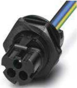
PRC device connector, black, 3-pos., 2.5 mm 2 /630 V/35 A, crimp connection, with 150 mm cable length, cut flat at the end
