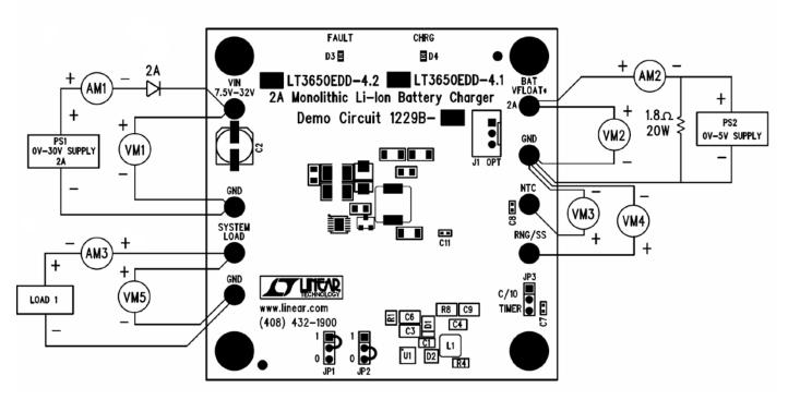
**Note:** Put a blocking diode between the input supply and the  $V_{\text{IN}}$  terminal. Kelvin connect the voltage meters directly to the board terminals as shown on the diagram. Use twisted pair input and output leads.
