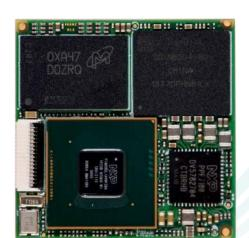
The i.MX 8XLite SoC based LGA Module is designed as per the Open Standard Module  $^{\text{TM}}$  specification (OSM). It integrates NXP's i.MX 8XLite offerings Dual/Solo Cortex A35 @ 1.2GHz, advanced multicore processing with V2X acceleration supported by Arm® cores.
