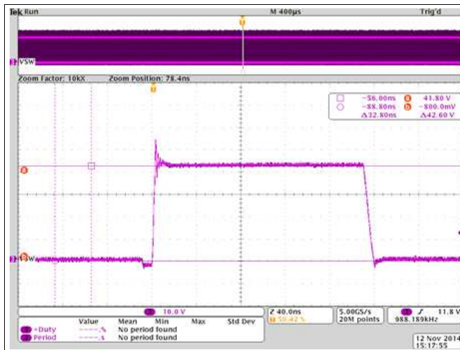
Figure 6. SW Node Behavior Showing the Dead Time and the Overshoot in the SW Node
