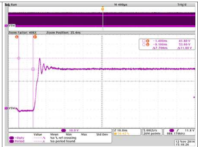
Figure 7. Zoom in of the SW Node Showing the Dead Time of 7.7 ns (Converter Loaded With 2 A)
