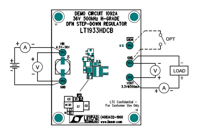
Figure 1. Proper Measurement Equipment Setup
