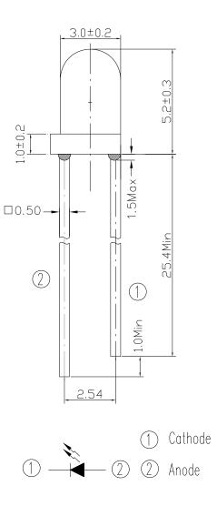
Note: Tolerances unless dimensions ±0.25mm
