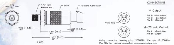
Vent through hole in connector ( under 1000 psi ) Add 0.4" for CE EMI/RFI protection. Note: Mating connector is available with 3 ft of cable PN (2001140).
