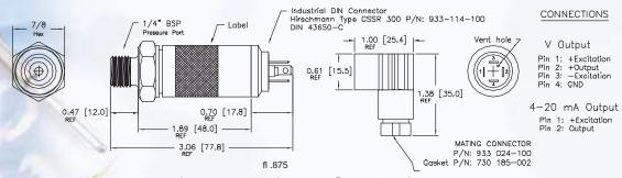
Vent through hole in connector ( under 1000 psi ) Add 0.4" for CE EMI/RFI protection.
