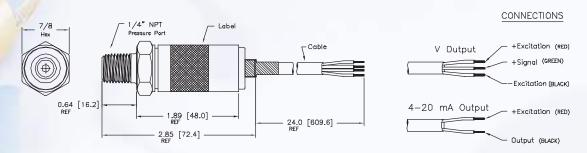
Vent through cable ( under 1000 psi ). Add 0.4" for CE EMI/RFI protection, max operating temperature for cable is 100°C.
