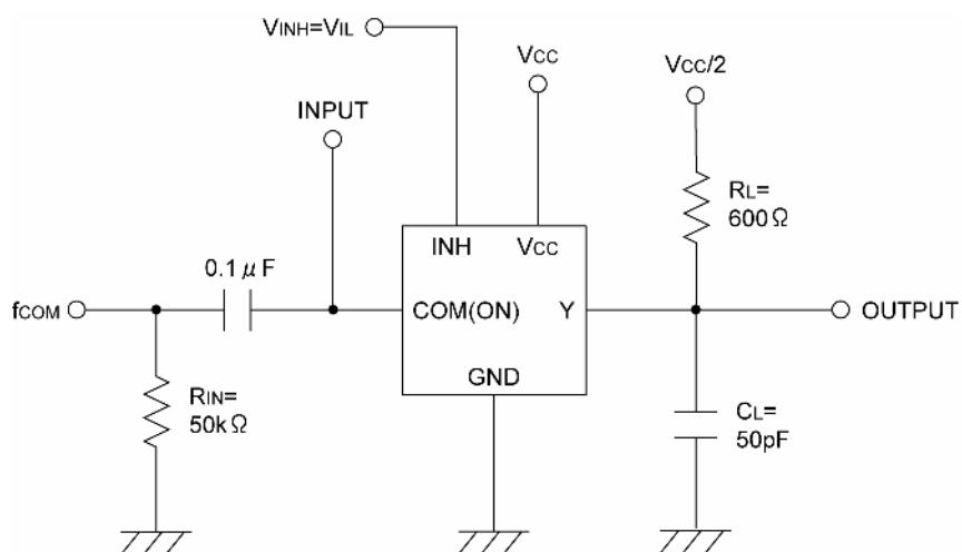
\* fCOM by sine wave( $V_{COM}=V_{CC}/10[V_{p-p}]$ )
